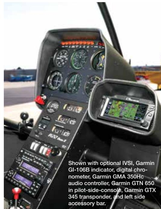
Shown with optional IVSI, Garmin GI-106B indicator, digital chronometer, Garmin GMA 350Hc audio controller, Garmin GTN 650 in pilot-side-console, Garmin GTX 345 transponder, and left side accessory bar.
