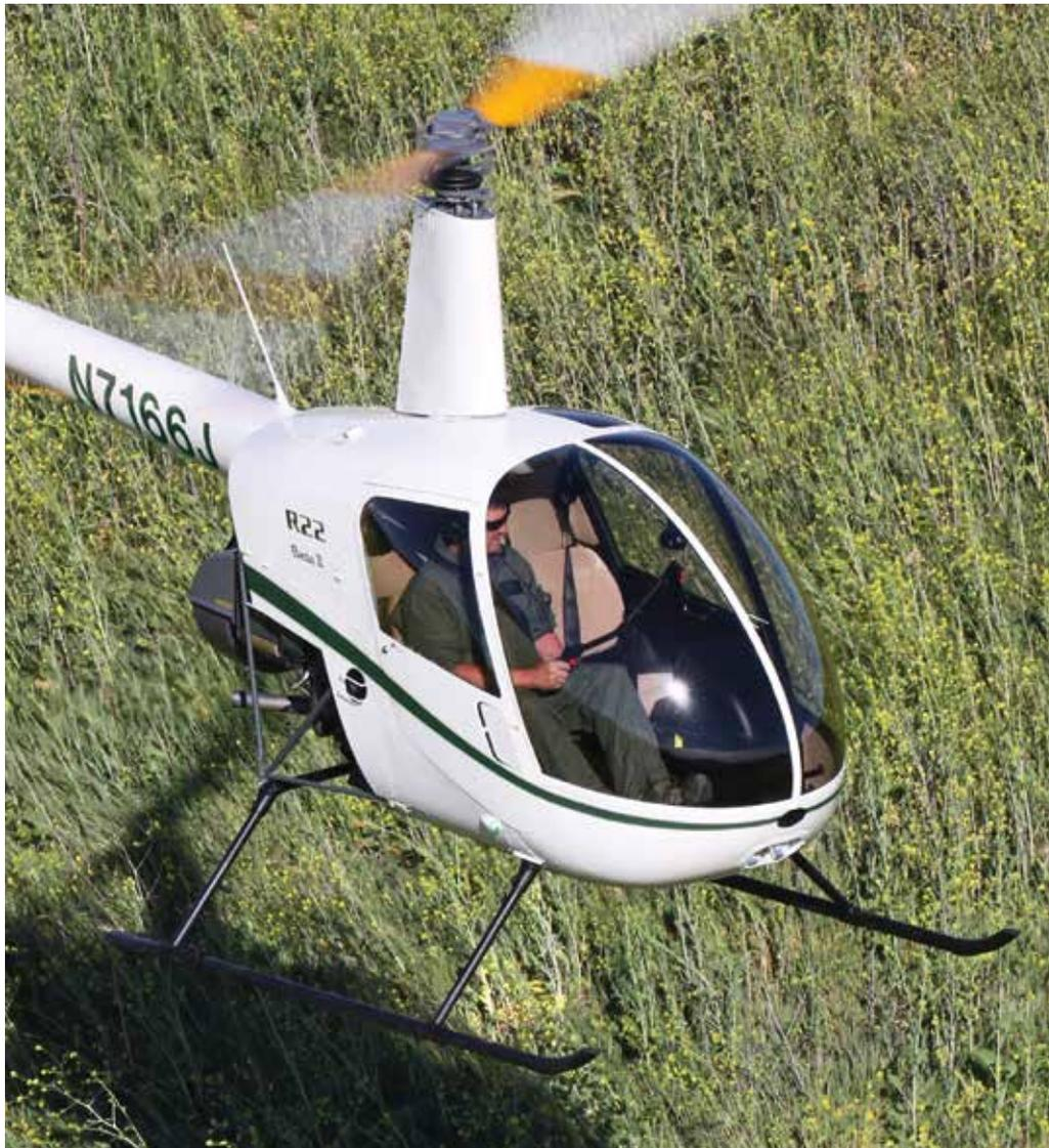
The two-seat R22 helicopter is a proven workhorse that has delivered exceptional performance in a variety of applications for over forty years. The R22 has a two-bladed rotor system which requires minimal hangar space, a T-bar cyclic for easy entry and exit, and a crashworthy fuel system.
