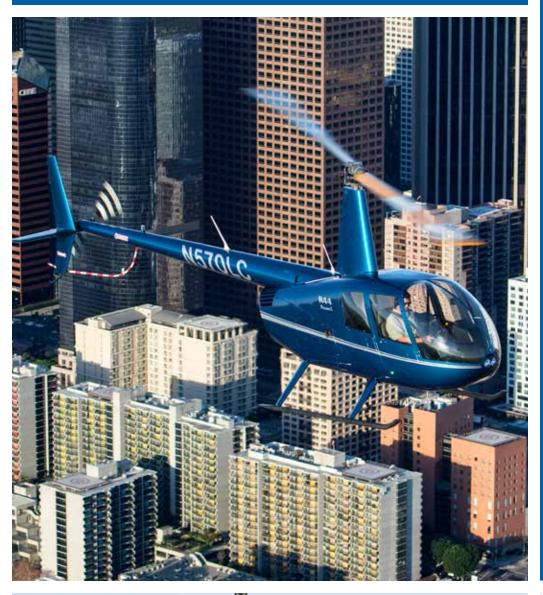
Four-seat R44 Raven I and Clipper I helicopters are high performing, reliable and easy to maintain. R44s have a two-bladed rotor system, T-bar cyclic and the latest in Robinson technology including streamlined instrument panels and crashworthy fuel bladders.
